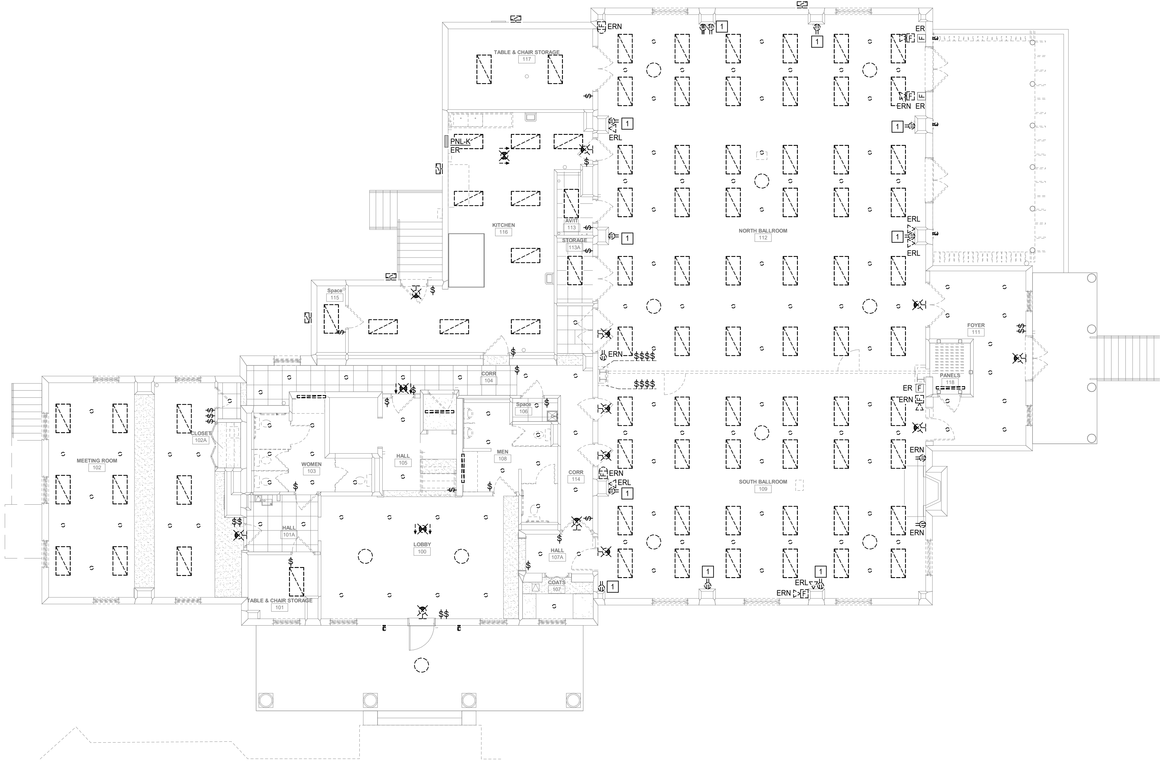
1 FIRST FLOOR ELECTRICAL DEMOLITION PLAN Scale: 1/8" = 1'-0"
